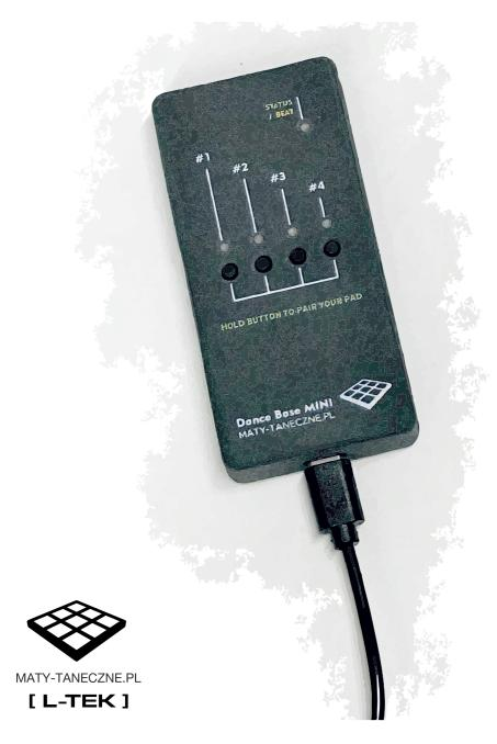
The STATUS LED on Base MINI lights up green after Base MINI is connected to the computer's USB port
